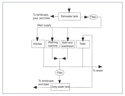
Figure 3. Integrated gray-water reuse system.
